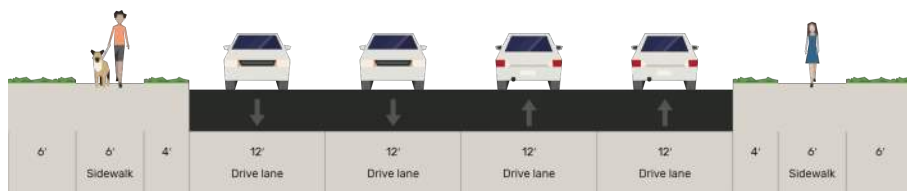
Exhibit 6.5: Major Collector Cross Section
