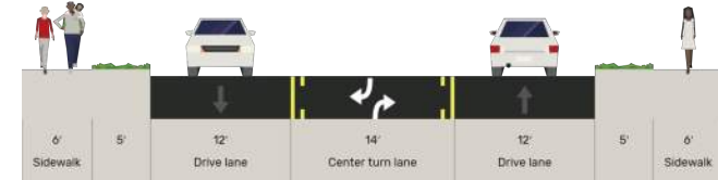
Exhibit 6.6: Minor Collector Cross Section
